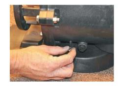
4. Make sure the pump is straight in the base and the screws are aligned vertical before tightening.
