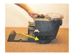
3. Place the stainless steel flat washers over the base flanges on each side of the pump. Insert the two stainless steel screws and start the two base mounting screws by hand.
