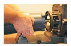
9. Slide the motor toward the pump until it touches the motor adapter.
